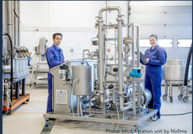
Photo: Microfiltration unit by Nofima
